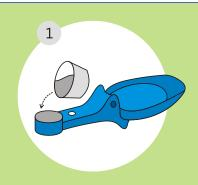
Fill the cup of Flap Door with sufficient cement paste
