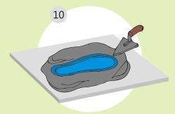
Spread the mixture of sand and cement paste
